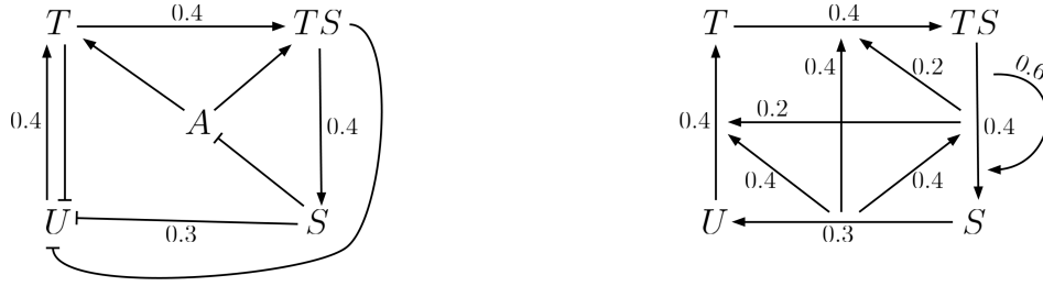
Figure 6.3: A graph diagram of circadian rhythm with some weights representing rates (left); and a complete weighted switch graph obtaining by removing inhibitor edges and component A (right).
