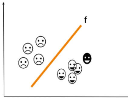
Figure 4.1.1: characteristic function f that correctly separates the two subsets of images, where white faces represent the training set, and the blackface represents a new face that f must be able to classify.
